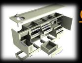
Construction system of base cabinets
